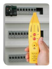
The Circuit breaker that supplies the Transmitter circuitry is the one, that (when pointed out by the tip) has the most LEDs lit on the bar-graph and the fastest audible alarm.
